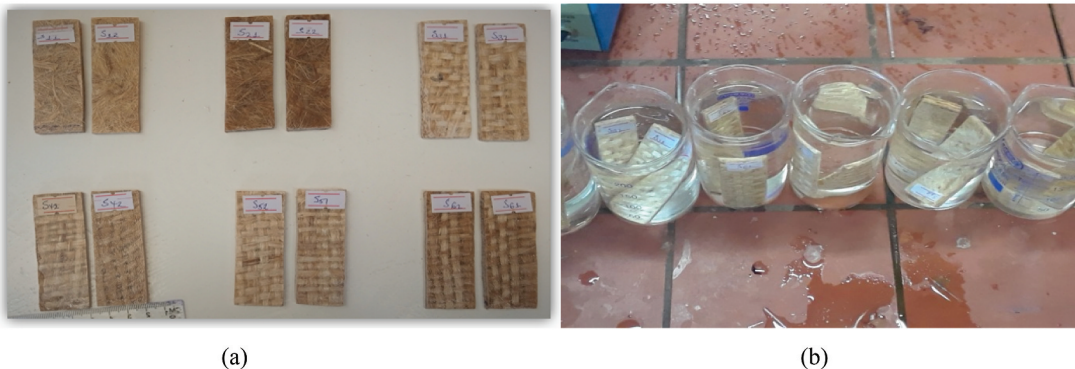
Figure 2. (a) Specimens for water absorption test and (b) specimens immersed under test.
