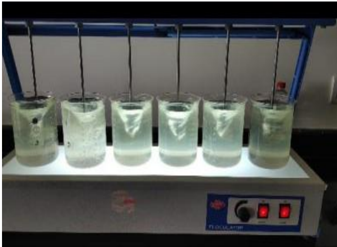
Figure 3: Jar test apparatus setup
