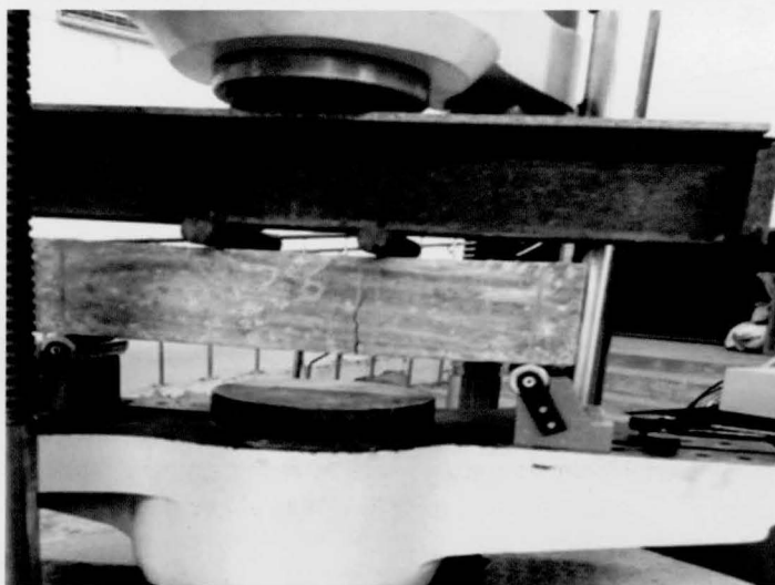
Figure 2: Flexural strength test arrangement.
