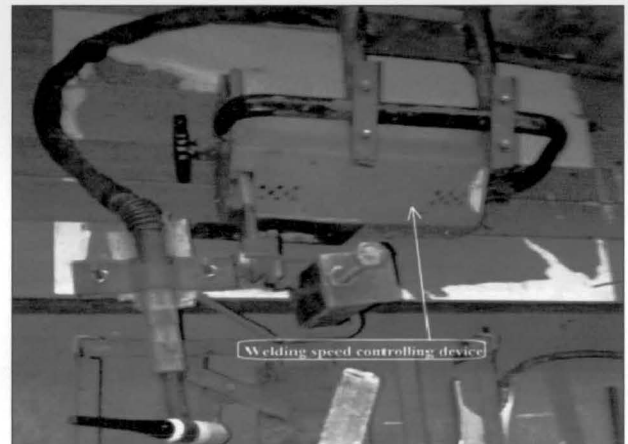
Fig. 3. Photograph of constant welding speed controlling device.
