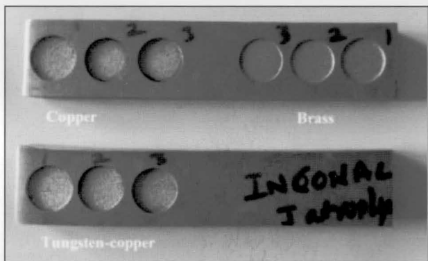
(c) Sample with Jatropha oil as dielectric fluid.
