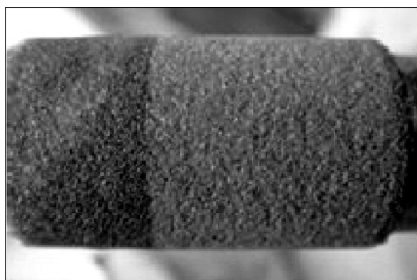
Fig 6. Laser Dressed Wheel with Loaded Portion
