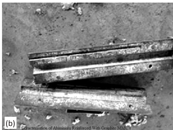
Fig 1. Die Used to Produce the Test Specimen
