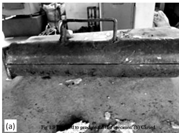
Fig 1. Die Used to Produce the Test Specimen
