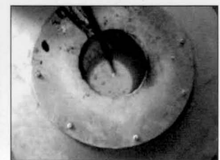
Fig 4.4. Molten Metal in furnace
