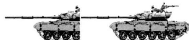
Fig. 13 Rarely seen microscanning artifact produced by observing target moving at extremely high angular rates.
