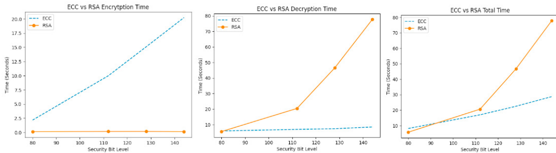
Fig. 7 (a) and (b). RSA vs ECC Encryption, Decryption and Total Time for 64-bit input
