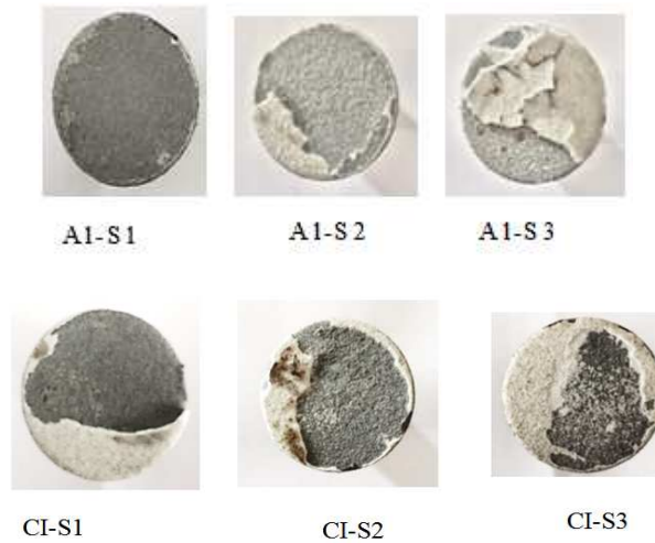
Figure 6: Fractured Surfaces of Adhesion Test Specimens
