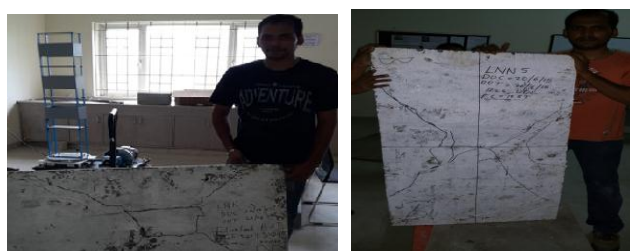
Crack pattern for S1 and S2 slabs
