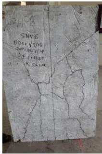
Crack pattern for S5 and S6 slabs
