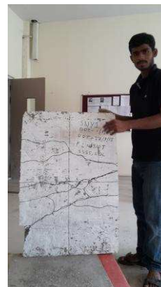
Crack pattern for S1 and S2 slabs
