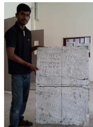
Crack pattern for S1 and S2 slabs
