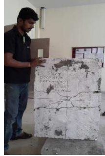
Crack pattern for S5 and S6 slabs
