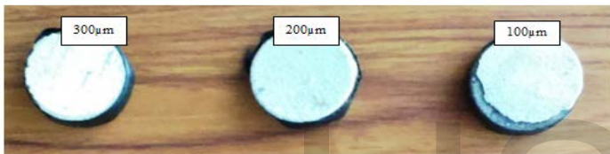
Fig-5: Images of the top coat samples under 10 % diluted HNO 3 solution after 24 hours.
