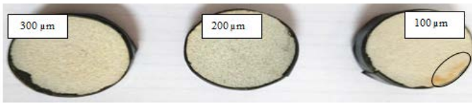
Fig-3: Images of the top coat samples under 5 % diluted HNO 3 solution after 24 hours.
