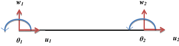
Figure 1: Two- node Euler–Bernoulli elements.
