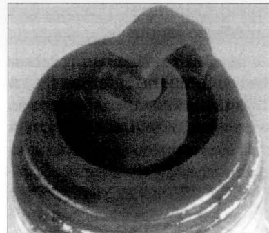
Fig. 3. Carbon deposited electric spark plug.
