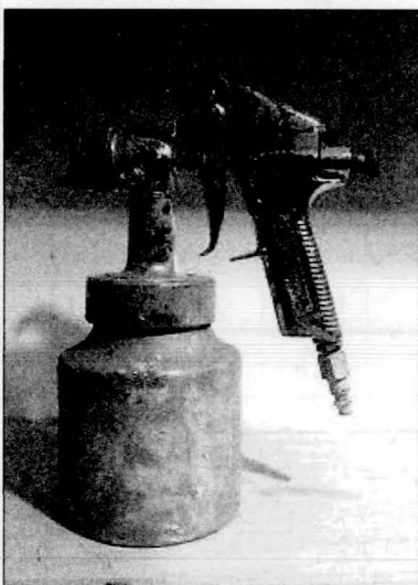
Fig. 4. HVLP spray gun used to spray LDAM.
